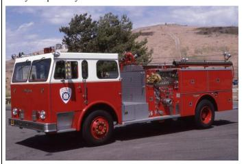
During a good portion of the decades of the 1960's and 70's both the Navy and Marine Corps Fire Departments were operating with two door tilt cab commercial chassis apparatus equipped with 750 gpm fire pumps and 300 gallon water tanks. While these pumpers typically built on either Chevy or GMC chassis
